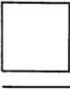
FIGURE 75. SYMBOLS for controlled dynamical systems may be made schematically by representing the control space as a horizontal line segment and the state space as a vertical line segment, regardless of the actual dimensions of these spaces. A single dynamical system with controls then is represented by a box with a line beneath it.
